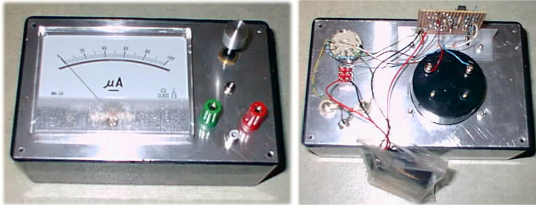
Figure 12 - The finished meter. The first image shows the front of the aluminium panel. The second image shows the back of the aluminium panel.
